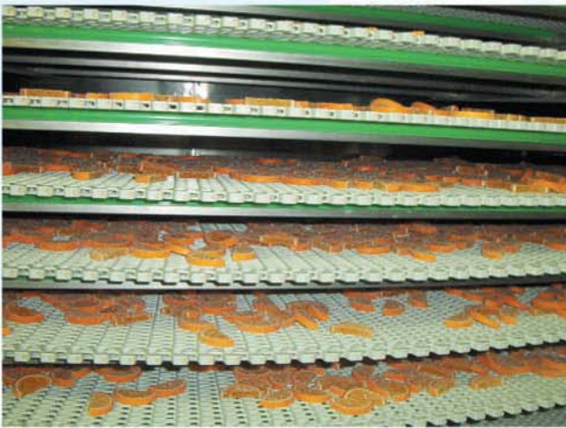
Schüttgut-Pufferung/buffering of bulk products
